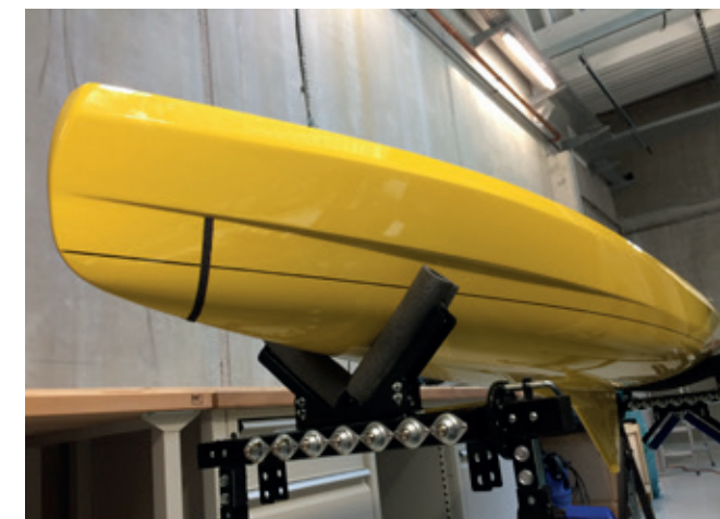
Model hull made by 3D printing process
